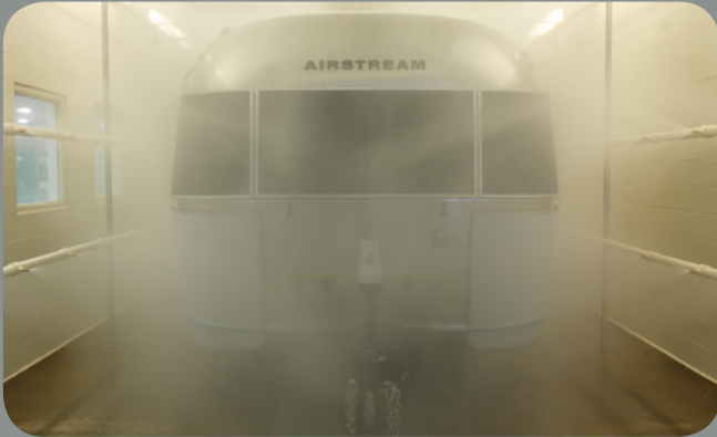
Every Airstream is subjected to extensive, high pressure water testing
