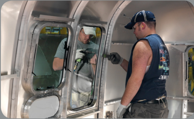
Over 3000 rivets are riveted into place by skilled specialists working in pairs
