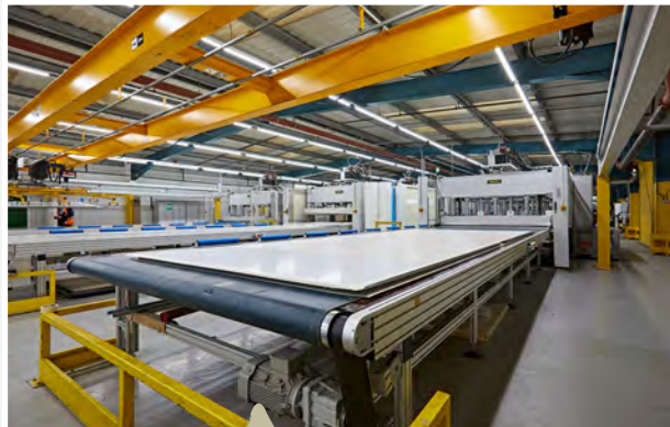
'SMART' GRP sidewall during the production process.
